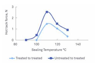
**Figure 4.** Effects of corona treatment on sealing. Attempting to seal two treated surfaces to each other results in lower hot tack strength and a narrow sealing temperature range.
