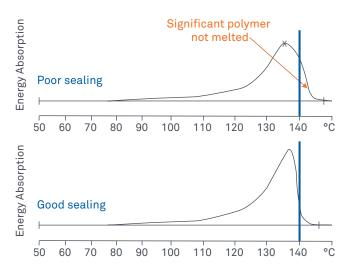
**Figure 8.** DSC curves show the amount of energy being used to melt the polymer over a temperature range. At any given temperature, a higher energy level indicates that more of the polymer is melting at that temperature.
